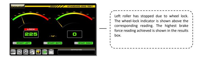
5. If wheel-lock cannot be reached while maximum brake force is being applied the rollers can be stopped by pressing the F1 key again (or any other key).
