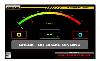
After the SERVICE BRAKE test, the software will re-start the rollers. The user is asked to CHECK FOR BRAKE BINDING. This message is shown for two seconds. There is no software measurement for brake binding and the user must make a note if present.
