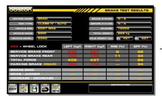
The test is now complete and the user is asked if there was any BIND, GRAB or JUDDER from any wheel during the test. If so, the user must select F1 and complete the page above. If not, then select F2 NO and the results page will be shown.
