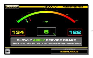
The software now checks for IMBALANCE. The user must SLOWLY APPLY THE SERVICE BRAKE until the force from either wheel reaches 75% of the maximum force achieved in the previous SERVICE BRAKE test. The red needle indicates this value and when reached, an audible bleep is sounded by the software. If wheel lock is achieved during this test the software automatically restarts the rollers.
