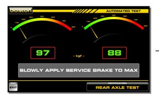
Once the PARKING BRAKE test is complete the software must check the SERVICE BRAKE. The software automatically restarts the rollers and instructs the user to SLOWLY APPLY SERVICE BRAKE TO MAX.
