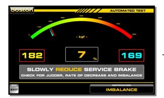
Once the force has reached 75% of the previous maximum, the message SLOWLY REDUCE SERVICE BRAKE is shown. The user must reduce brake effort and the software will automatically turn off the rollers when the brake force falls below 40kgf.
