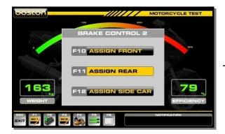
ASSIGN rear wheel brake force measurement from brake control 2 to the REAR.
