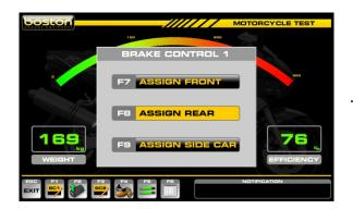
Assign REAR wheel result to BC1 when FIRST brake control operates on the REAR wheel.
