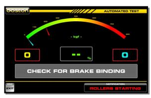
After the SERVICE BRAKE test, the software will re-start the rollers. The user is asked to CHECK FOR BRAKE BINDING. This message is shown for two seconds. There is no software measurement for brake binding and the user must make a note if present.
