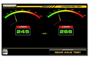
If wheel lock is achieved, the LEFT and RIGHT indicators will show. If wheel lock cannot be achieved, the software will automatically stop the rollers when stable readings have been measured for 3 seconds.
