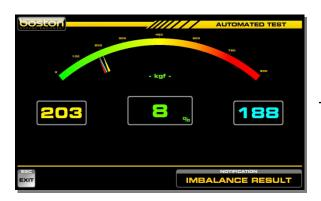
After the rollers have stopped, the IMBALANCE result is shown for a few seconds before the software completes the test.
