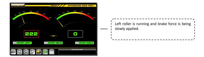
4. Continue to apply brake force until maximum force or wheel-lock is achieved. If wheel- lock occurs a red indicator will be shown on the display. At the point where the tyre slips on the roller the motor will be stopped immediately to avoid unnecessary tyre wear.
