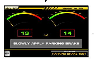
After centralising the wheels, the operator is prompted to SLOWLY APPLY PARKING BRAKE.
