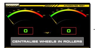
The rollers will start automatically and the operator is prompted to centralise the wheels in the rollers. This message is shown for 2 seconds.
