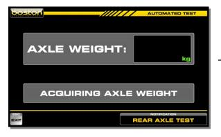
The axle is weighed automatically. This page is shown for approximately 4 seconds. The axle weight is then shown.
