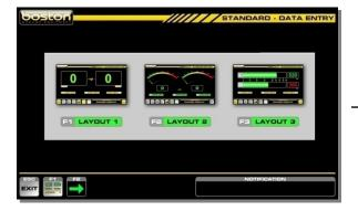
Using the mouse, keyboard or remote control, select F1, F2 or F3 to choose a layout. The chosen layout will be shown on the first measurement screen after the vehicle has been placed in the rollers.
