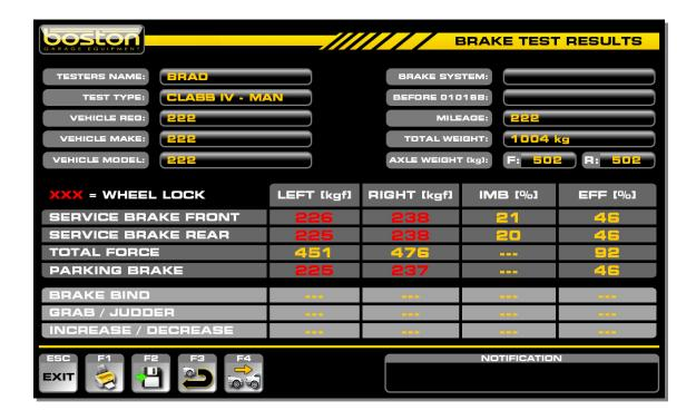
If the user correctly saved the data for each wheel during the test, the software will automatically calculate the brake efficiencies for the front and rear axles. For AUTOMATED tests, the software stores the results automatically during the test and produces a PASS / FAIL result.
