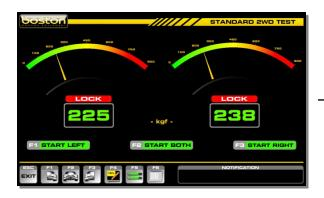
Even though the RIGHT wheel was tested, the result for the LEFT wheel still remains shown for comparison. The right wheel result is shown in the corresponding result box.
