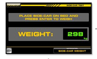
Place sidecar on the bed and wait for the weight reading to become stable. Press ENTER to assign the weight.
