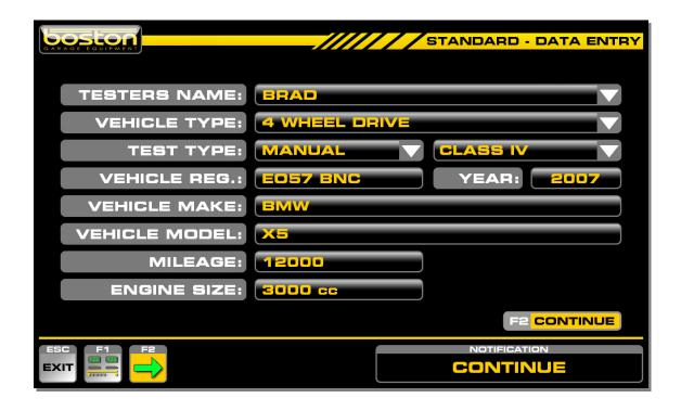
Complete the DATA ENTRY page as before but select 4 WHEEL DRIVE as the vehicle type. The TEST TYPE will be set to MANUAL. Select F2 CONTINUE.
