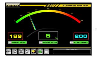
The rollers have started and brake effort is gradually applied. Both readings for LEFT and RIGHT can be seen together in both digital and analogue format using two different colour needle pointers. This gives a good indication of severe imbalance if present.
