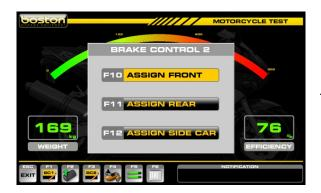
Assign FRONT wheel result to BC2 when SECOND brake control operates on the FRONT wheel.
