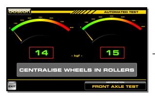
The message CENTRALISE WHEELS IN ROLLERS is shown for 2 seconds, the operator is then prompted to slowly apply the service brake to maximum.
