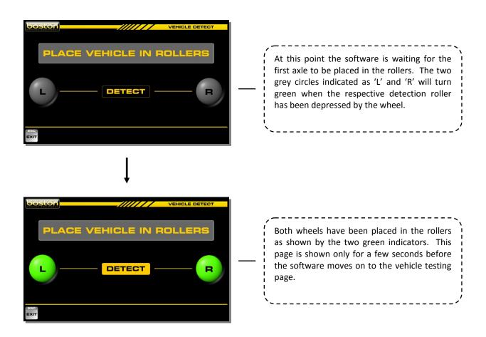
Once the rollers have been depressed, the detect indicators turn green and the software enters into the vehicle testing page. From this point onwards the testing procedures may differ depending on the vehicle details entered on the DATA ENTRY page.
