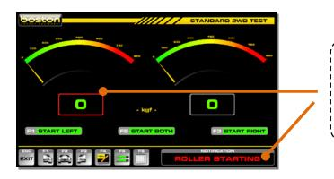
In this example, the left roller has been selected. There is an audible buzzer and three flashes of the red box to alert the user. The message 'ROLLER STARTING' is also shown in the notification box.
