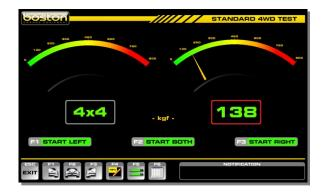
During the testing of the FRONT RIGHT wheel, the text 4x4 is shown in the left side results box. The left side roller is also operating but in the reverse direction. In this display layout, the analogue needle pointer is removed from the inactive measurement display.
