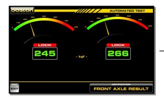
If wheel lock is achieved, the LEFT and RIGHT indicators will show. If wheel lock cannot be achieved, the software will automatically stop the rollers when stable readings have been measured for 3 seconds.
