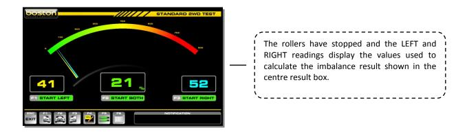
After the rollers have stopped, the results of maximum IMBALANCE achieved throughout the test are shown on the display. The readings shown are those which were used to calculate the imbalance percentage as shown in the centre result box. Refer to Chapter 5 for permissible limits.
