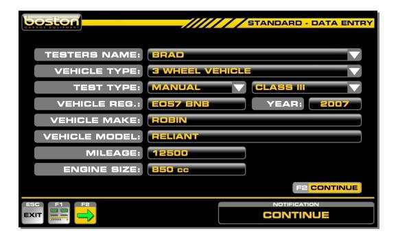
Complete the DATA ENTRY page as before but select 3 WHEEL VEHICLE as the vehicle type. The TEST TYPE will be set to MANUAL and the class of test to CLASS III as default. The user can also set the class of test to CLASS IV should the weight of the unladen vehicle exceed 450kg. Select CONTINUE.
