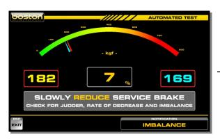
Once the force has reached 75% of the previous maximum, the message SLOWLY REDUCE SERVICE BRAKE is shown. The user must reduce brake effort and the software will automatically turn off the rollers when the brake force falls below 40kgf.
