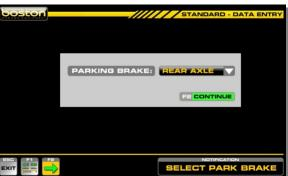
The next page asks the user to confirm the location of the PARKING BRAKE. This is usually fitted to the REAR axle and the software defaults to REAR. However, if it is fitted to the FRONT axle then select it here. The AUTOMATED procedure is different for each option.
