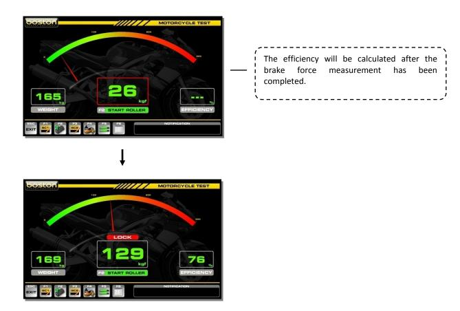
Once the brake force reading has been taken, the user must assign the result to memory. Select F1 or F3 depending on which brake control was used. For this example we will assume this test is the FRONT wheel using the HAND brake control BC1.
