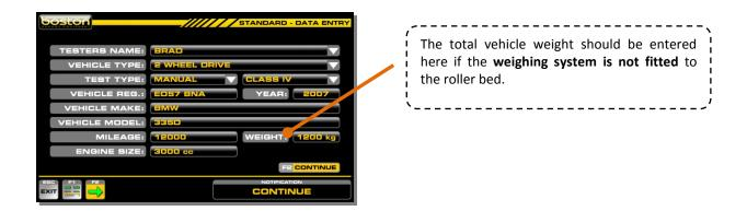
The software will acquire the axle weight automatically when the user starts either roller for the first time for each axle. The message ACQUIRING AXLE WEIGHT is shown while the system checks for a stable weight. The acquired axle weight is shown shortly after. See screenshots below in sequence. Once the weight has been acquired the software reverts back to the testing page and the selected roller(s) will start. There is an audible warning and warning text in red to alert the user.
