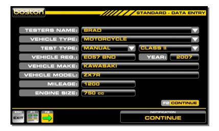
Complete the DATA ENTRY page as before but select MOTORCYCLE as the vehicle type. The TEST TYPE will be set to MANUAL and the class of test to CLASS II. Select CONTINUE.
