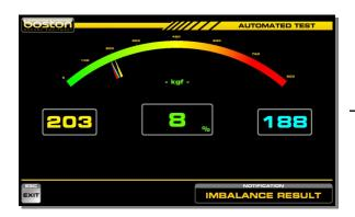
After the rollers have stopped, the IMBALANCE result is shown for a few seconds before the software moves on to test the rear wheels.
