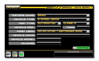
From this page the user selects the type of test required. If the relevant hardware and software is installed the software will continue into the respective program, if not, the message 'ACTIVATION REQUIRED' is shown. Similarly, if no tester's names have been set, the message 'SET TESTERS NAMES' will be shown.
