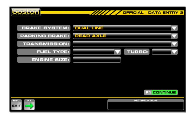
The compulsory fields are already completed by the software as default and the user can select F1-CONTINUE if the data is correct for the vehicle being tested.
