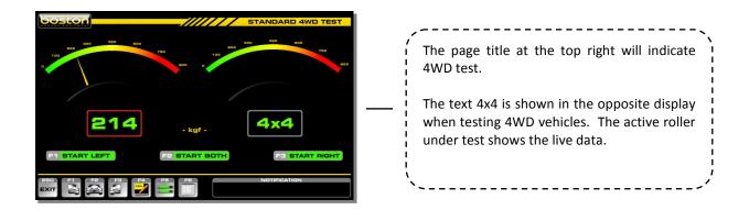
During the testing of the FRONT LEFT wheel, the text 4x4 is shown in the right side results box. The right side roller is also operating but in the reverse direction.
