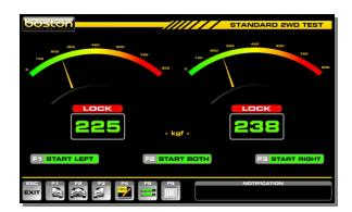
As we are now testing using the OFFICIAL TESTS procedure, when the user selects F6 RESULTS, a different page is shown that allows the user to enter BIND, GRAB or JUDDER for each wheel.
