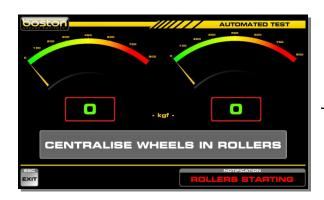
The rollers will start automatically and the operator is prompted to CENTRALISE WHEELS IN ROLLERS. This message is shown for 2 seconds.
