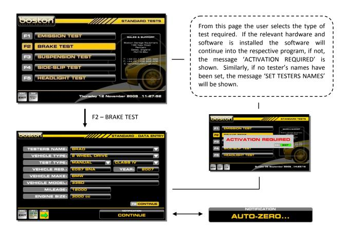
Whenever the DATA ENTRY page is entered, the message AUTO-ZERO will be shown briefly in the NOTIFICATION box. Whichever item of equipment has been selected from the test selection menu will be 'zeroed' prior to carrying out the test. At this point, it is important that the roller bed is clear and the roller covers are removed. If not, the software will 'zero' the system with an inaccurate measurement.
