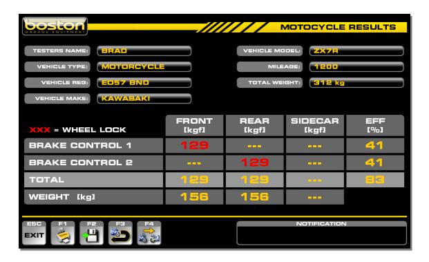
The screenshot below shows the same results page as above but with the added weight of the sidecar. With the added weight, we can see how the efficiencies have changed.
