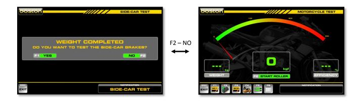
After the sidecar weight has been acquired, the operator can choose to test the sidecar brake (if fitted and controlled by either BC1 or BC2).
